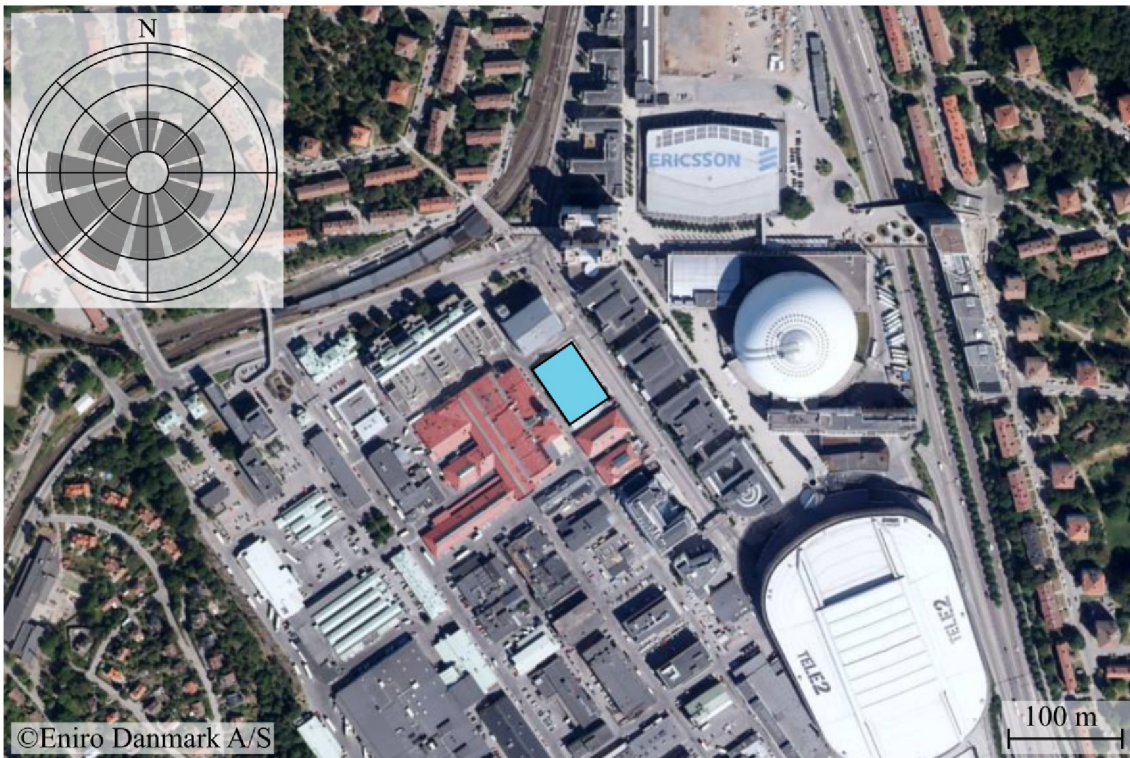
Figure 2. Aerial photo of the area with a blue rectangle indicating the location of the building at Sandhagen 2 and a wind rose for the Stockholm area indicating qualitatively that winds from southeasterly directions are the most frequent.
