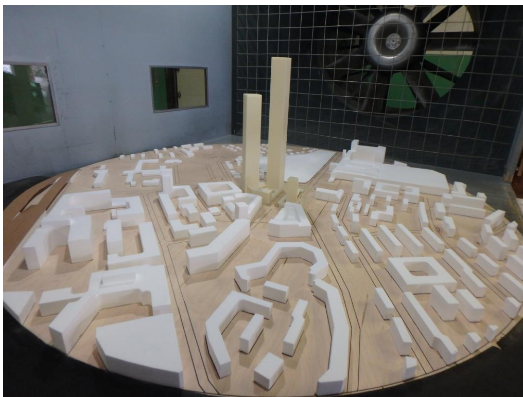
PHOTOGRAPH 1: STUDY MODEL INSIDE THE GWE WIND TUNNEL LOOKING DOWNWIND
